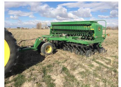
Direct Seed Drill planting directly into stubble from previous harvest.
