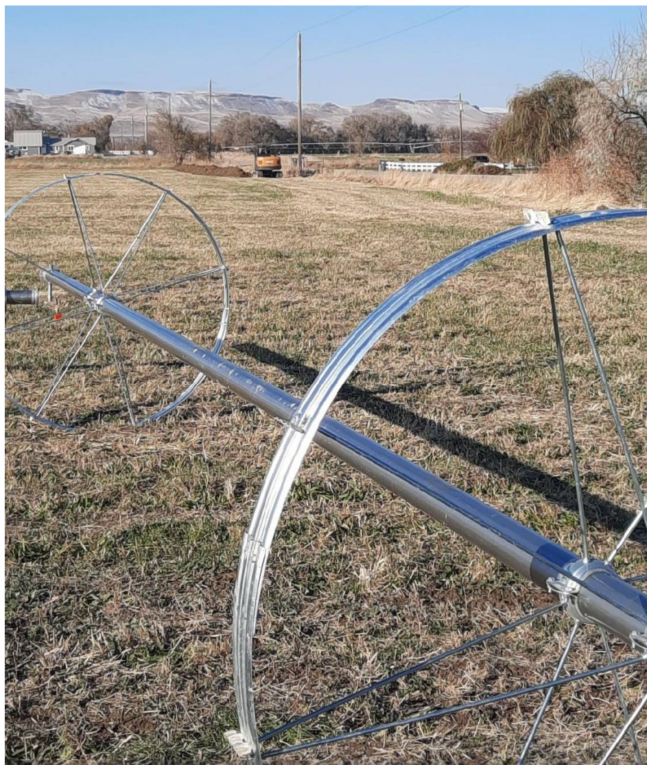
New irrigation wheel lines replace an old flood irrigation system on John Cossel’s hay farm near Jump Creek. (courtesy Owyhee District)
