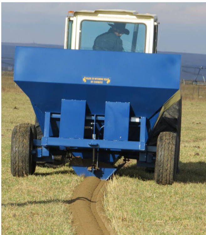
Left, Oteco pivot track filler in action. Right, pressurized irrigation system on the 26.9 Lateral canal provides a turnout at farm fields with pressure-relief valves and air vents to protect the new pipeline (courtesy Owyhee District).
