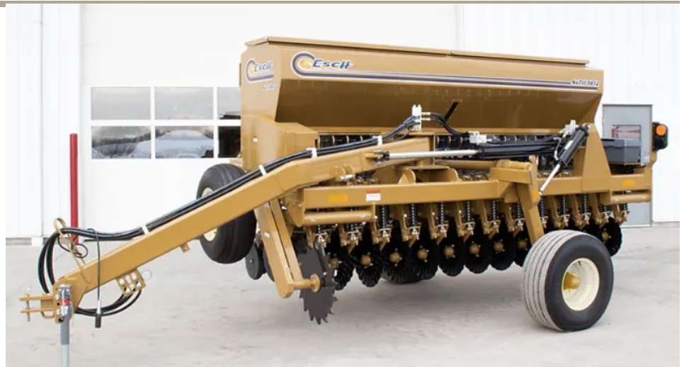
Kootenai-Shoshone SWCD is purchasing an Esch Model 5612, 12-foot no-till drill, which can be towed by a 80-100 HP tractor or a 3/4 to 1 ton pickup. (courtesy Jenna Ditzel/SWC)
