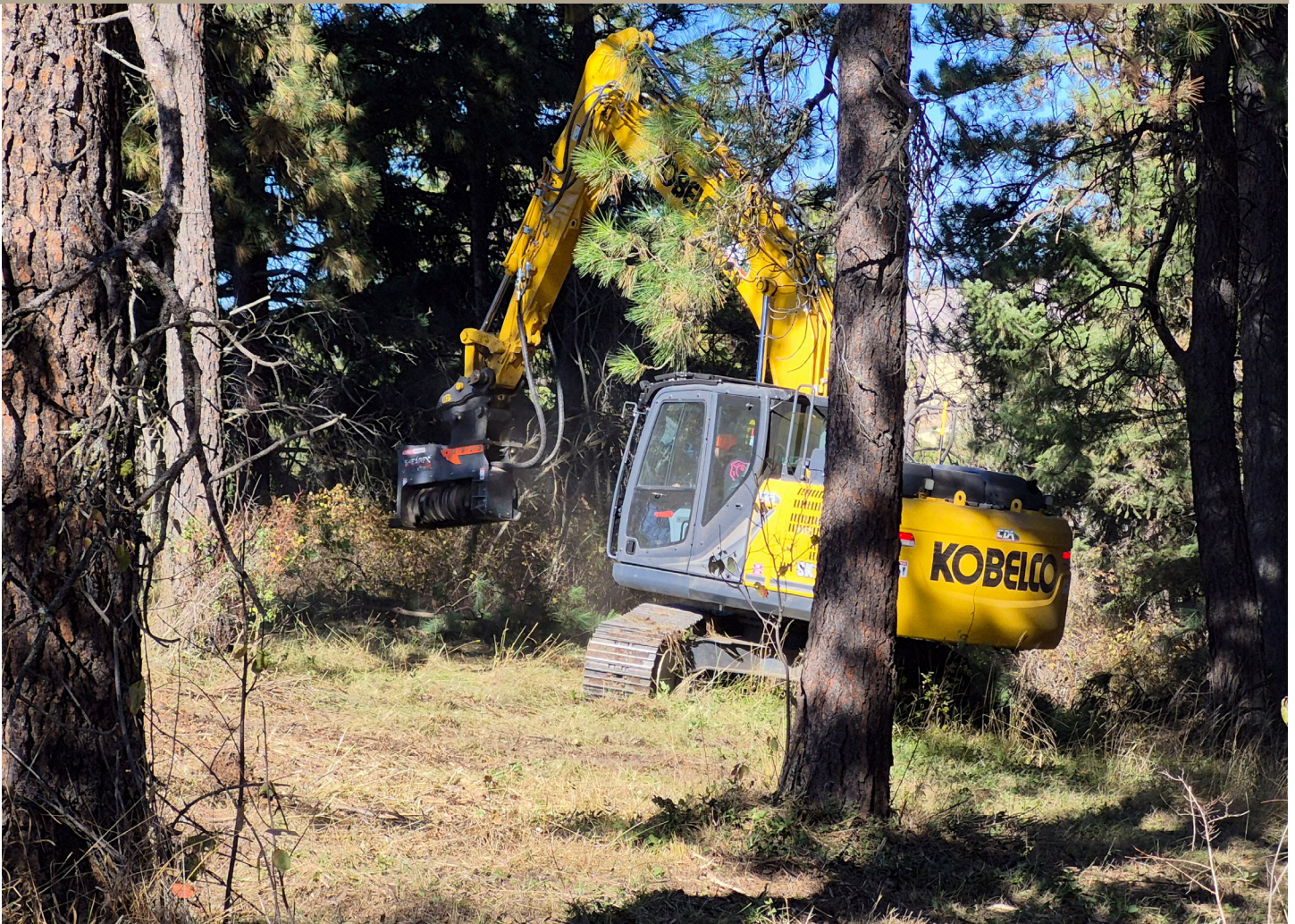
Masticator operator treats a brush patch at the Virgil Phillips Farm Park near Moscow this fall. The fuels-reduction project, sponsored by the Latah Soil and Water Conservation District and Latah County, will increase the park's resiliency from wildfire. (Photo courtesy Latah County)
