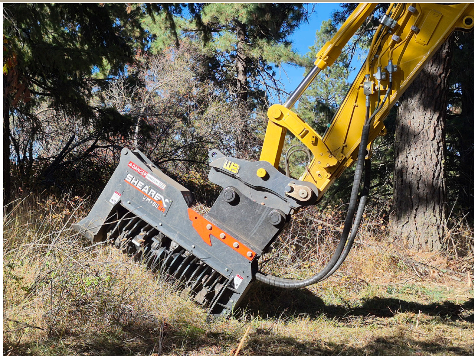
Trees and brush cut by the masticator were chipped and left on site to slow undergrowth, reduce maintenance, suppress weeds and control erosion. (photo courtesy Latah County)
