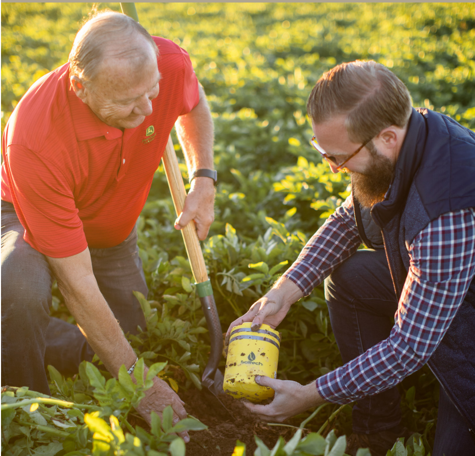
Moisture monitors should be buried about 6"-8" in a field so they can detect moisture, humidity and temperature in the plant root zone. (Soiltech photo)
